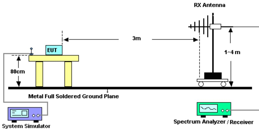
**For radiated test above 1GHz**
