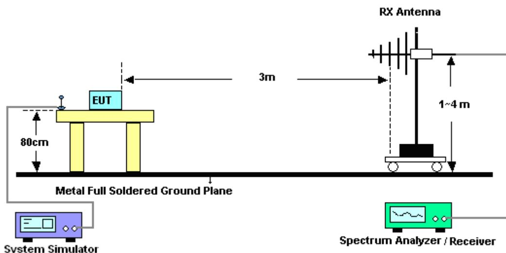
**For radiated test above 1GHz**
