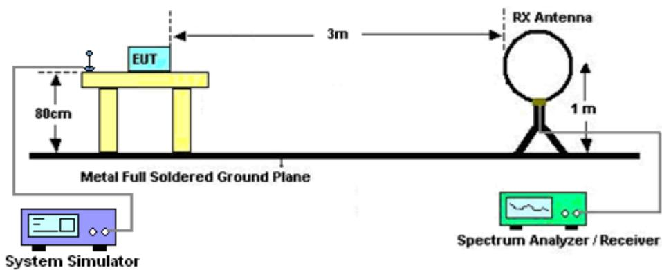
For radiated emissions from 30MHz to 1GHz
