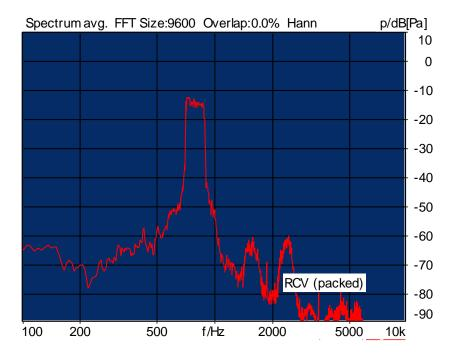
Distortion (Noise) RCV (packed): 35.55 dB (1.67%) Ok
