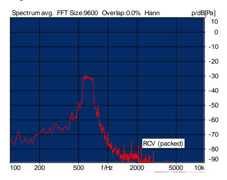
Distortion (Noise) RCV (packed): 24.27 dB (6.12%) Ok
