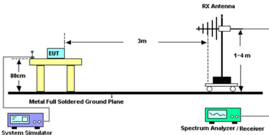
For radiated emissions from 1GHz to 18GHz
