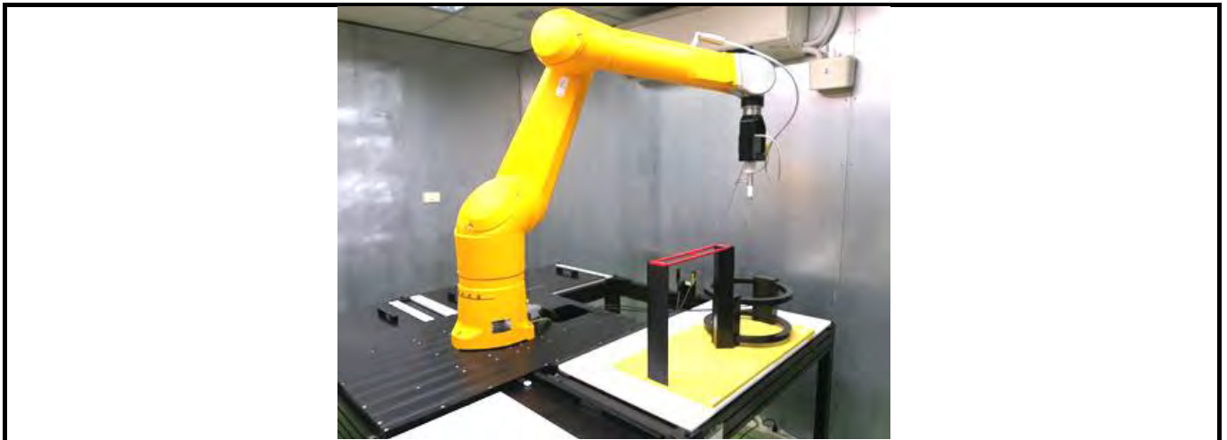
Fig-3.2 DASY52 Measurement System
