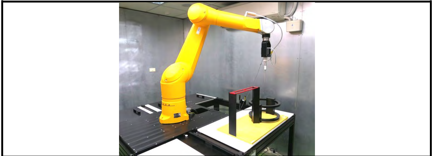
Fig-3.2 DASY52 Measurement System
