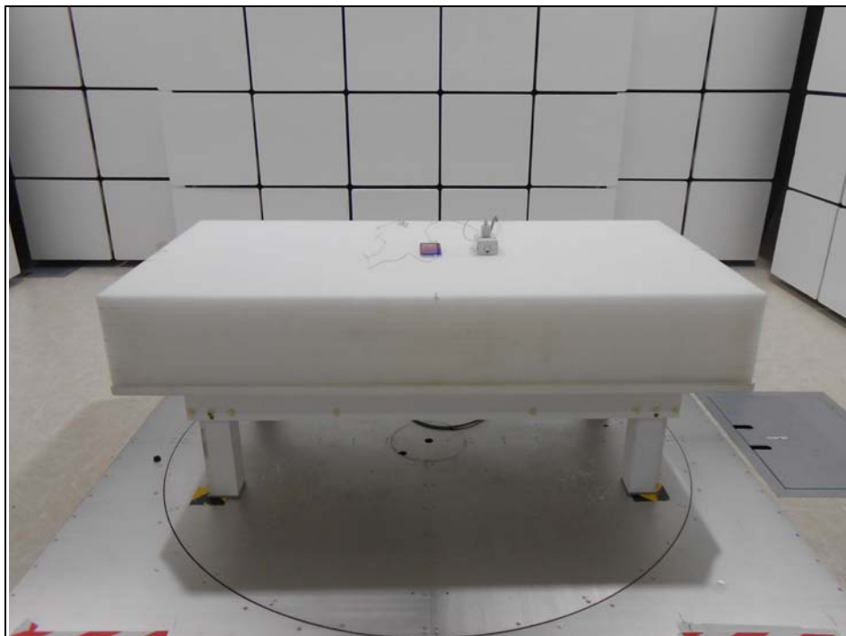
Radiated Emission Test (Below 1GHz) (X-plane)
