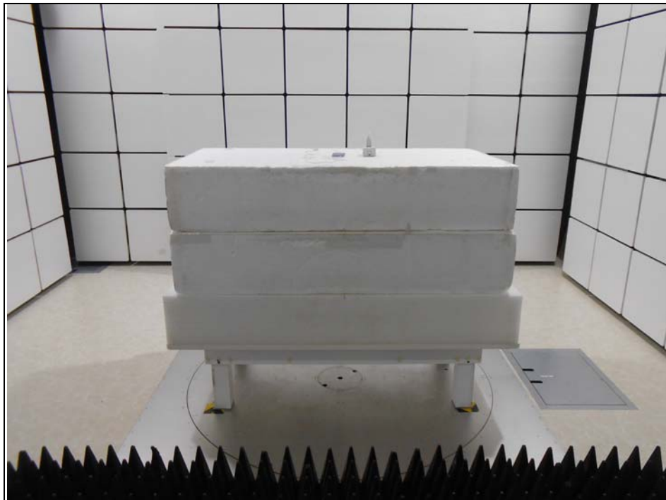
Radiated Emission Test (Above 1GHz) (X-plane)
