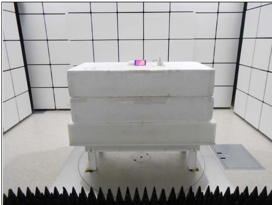
Radiated Emission Test (Above 1GHz) (Z-plane)
