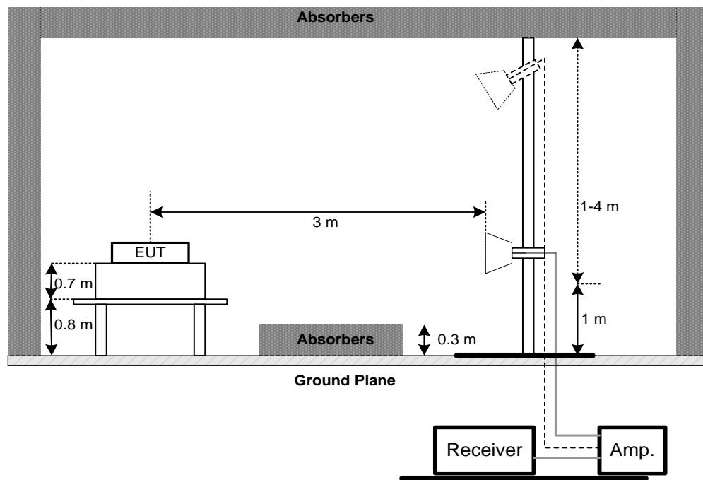
(C) For Radiated Emissions Below 30MHz
