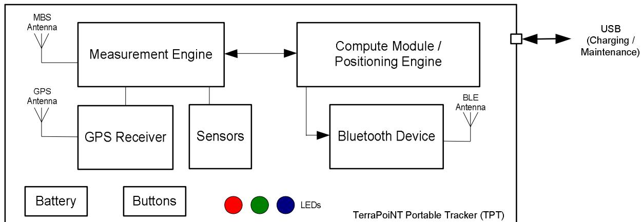
The TPT receiver system comprises of a measurement engine (ME) block, a compute module block, gps receiver and different sensors. The measurement engine block performs the acquisition and tracking of MBS beacon signals. The compute module receives the ME data and computes the ranges and trilateration to produce location fixes at 10Hz rate. The receiver is designed to interact and deliver location fixes to a host platform (Smart Phone) via Bluetooth.
