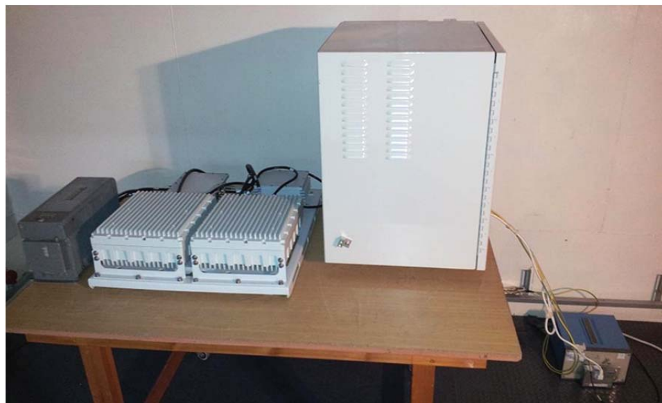
Photograph 8.1.1 Setup for conducted emission measurements
