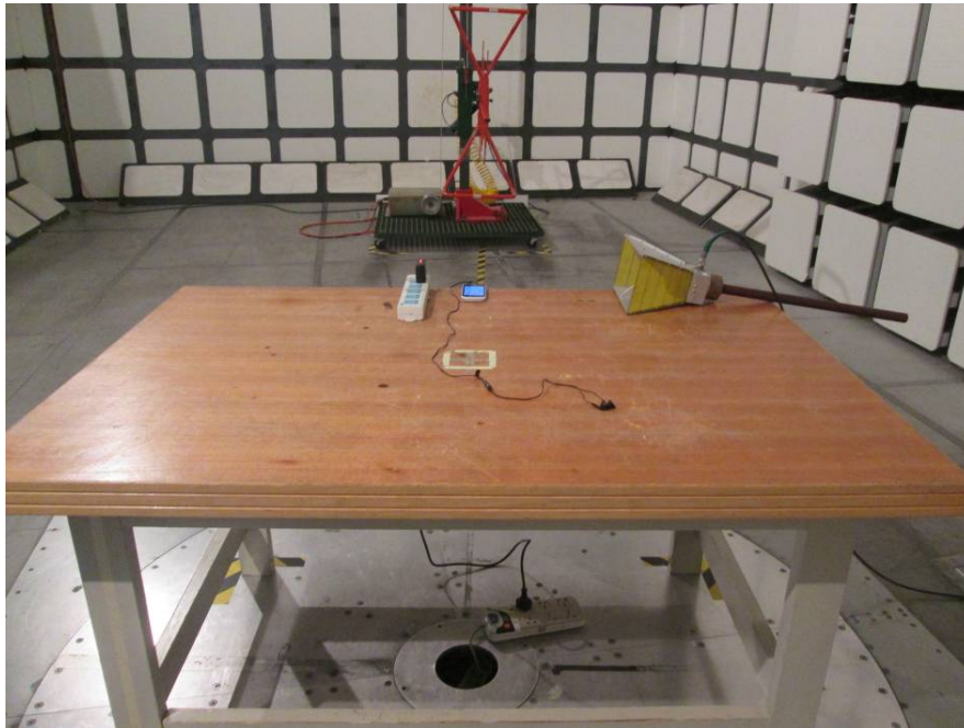
Radiated Emissions - Front View (Below 1 GHz)
