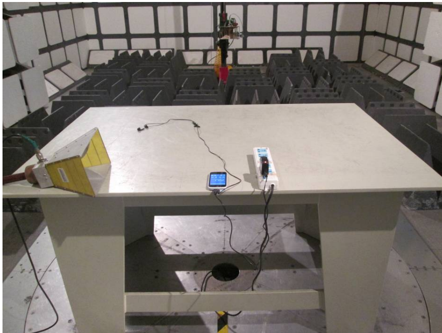
Radiated Emissions - Rear View (Above 1 GHz)
