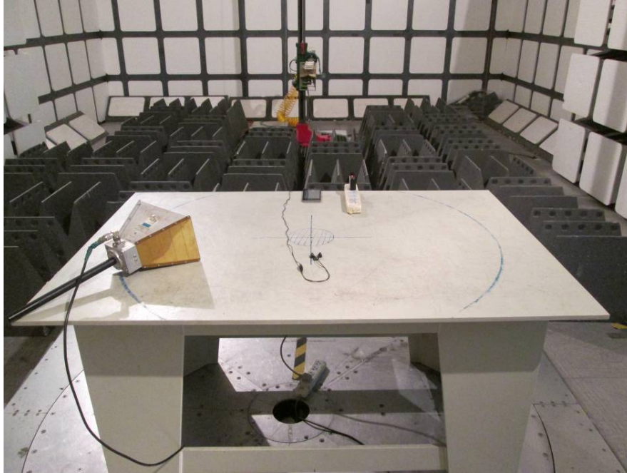
Radiated Emissions – Front View (1-25 GHz)
