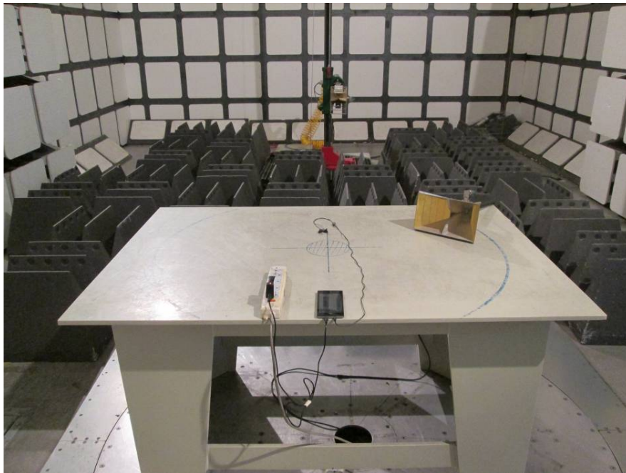
Radiated Emissions – Rear View (1-25 GHz)
