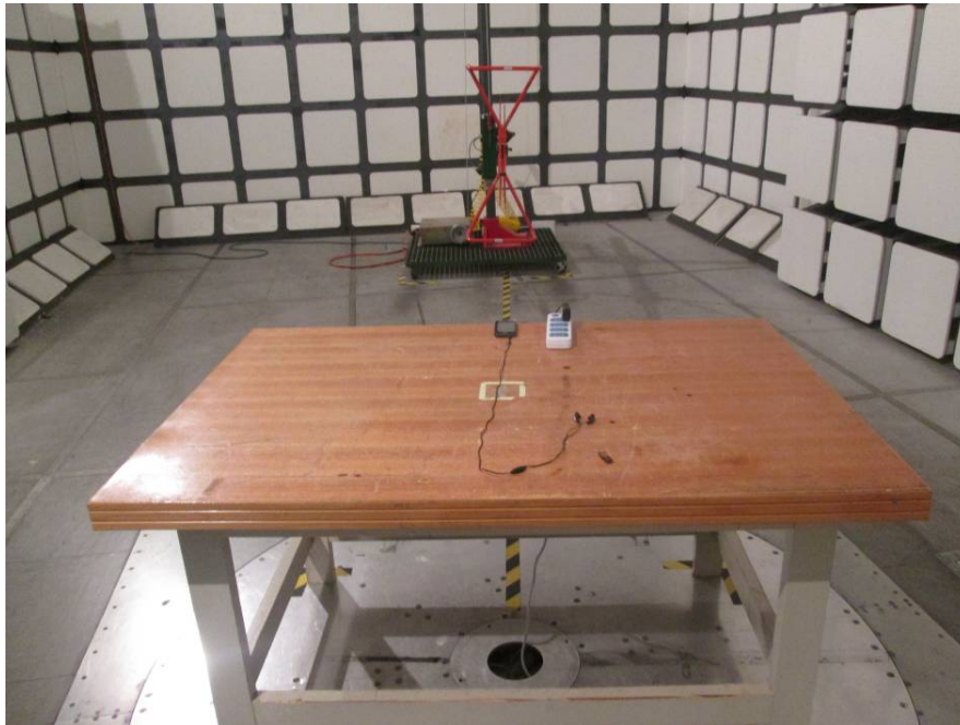
Radiated Emissions – Front View (30-1000 MHz)
