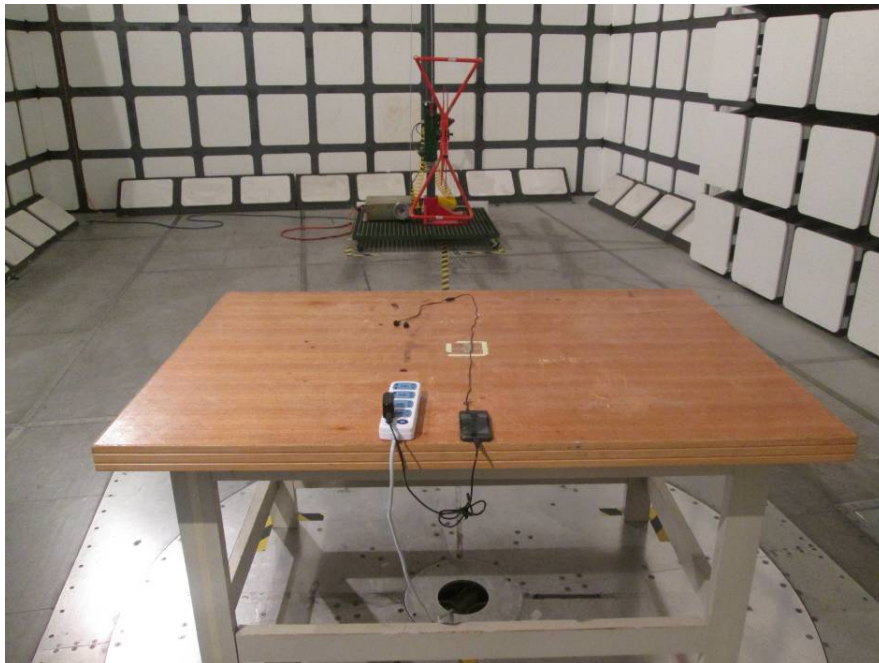
Radiated Emissions – Rear View (30-1000 MHz)
