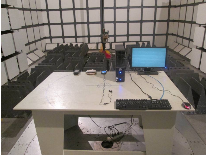
Radiated Emissions – Front View (Above 1 GHz)
