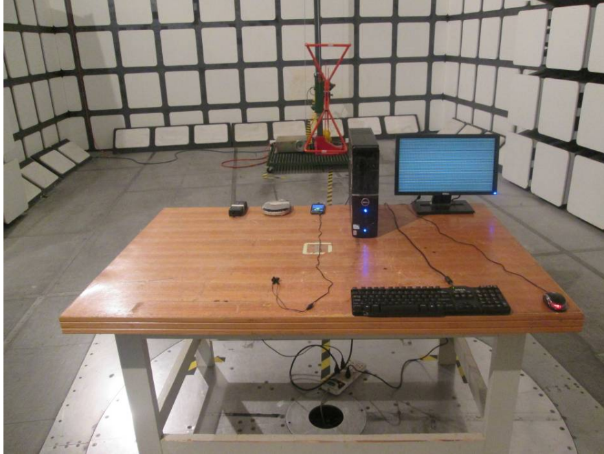
Radiated Emissions – Front View (Below 1 GHz)
