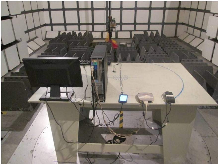
Radiated Emissions – Rear View (Above 1 GHz)
