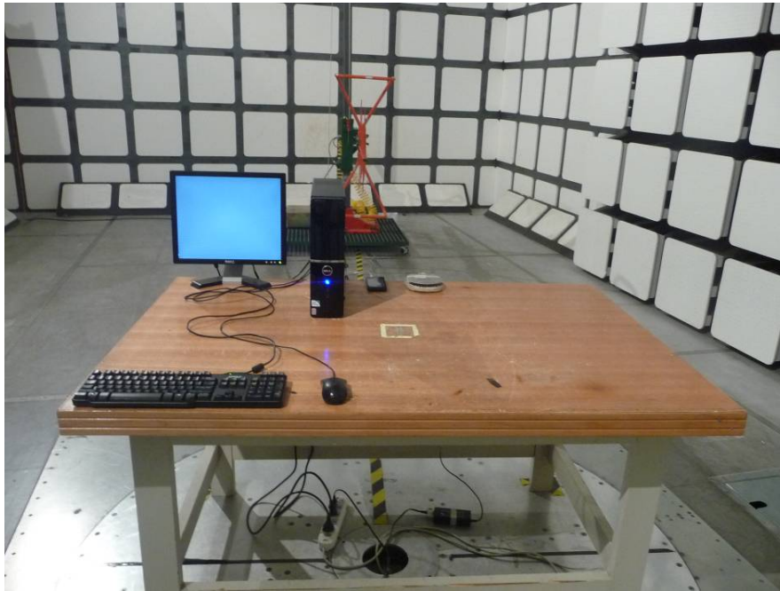
Radiated Emissions – Front View (Below 1 GHz)
