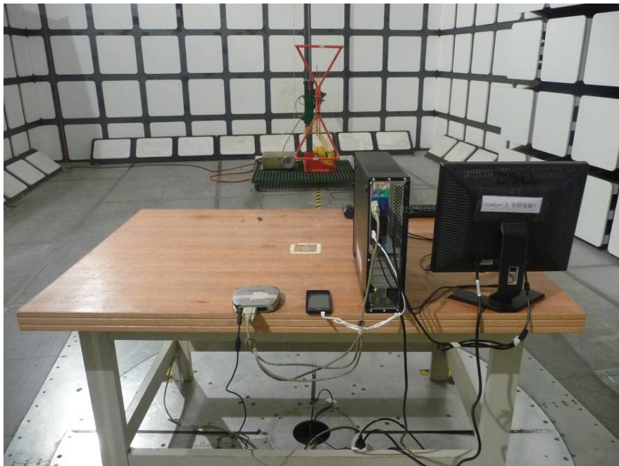
Radiated Emissions – Rear View (Below 1 GHz)
