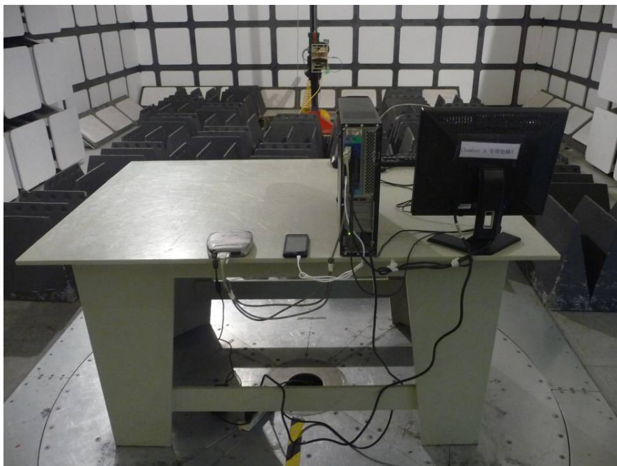
Radiated Emissions – Rear View (Above 1 GHz)
