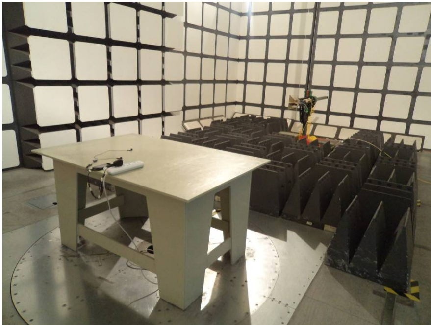
Radiated Emissions – Rear View (1-25 GHz)
