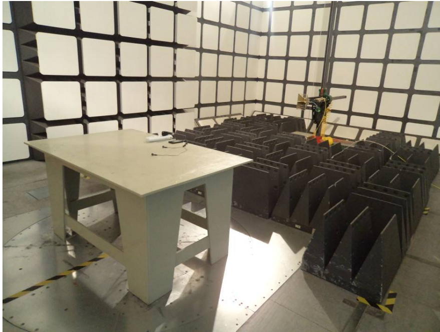
Radiated Emissions – Front View (1-25 GHz)
