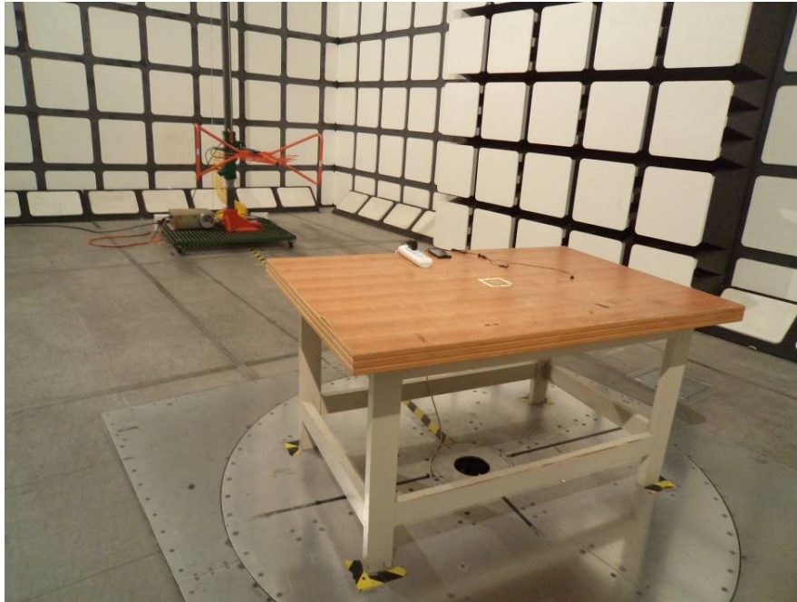
Radiated Emissions – Front View (30-1000 MHz)
