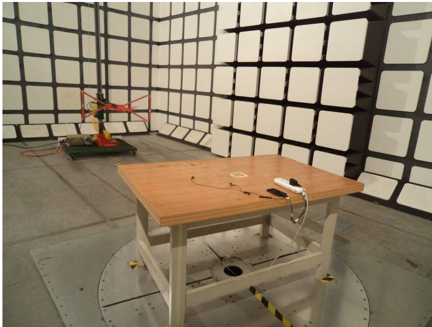
Radiated Emissions – Rear View (30-1000 MHz)
