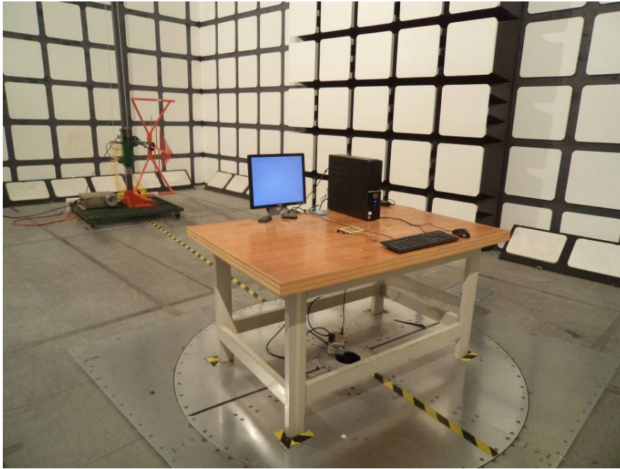
Radiated Emissions – Front View (Below 1 GHz)
