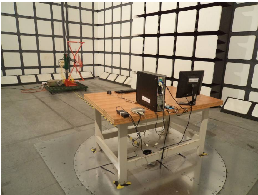
Radiated Emissions – Rear View (Below 1 GHz)
