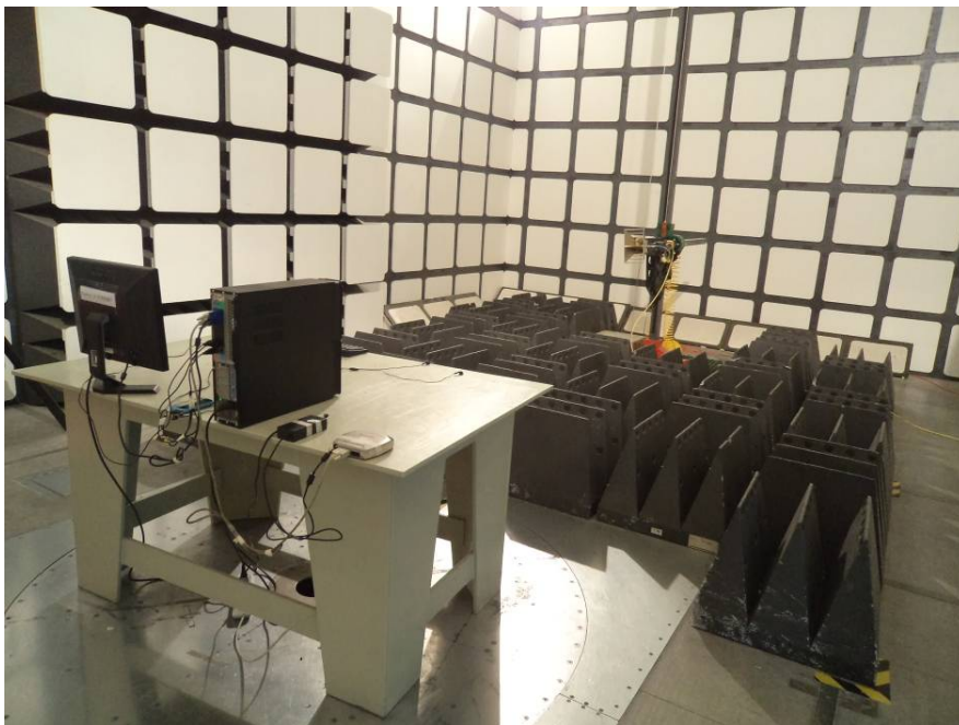
Radiated Emissions – Rear View (Above 1 GHz)
