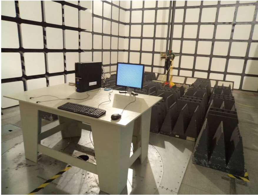
Radiated Emissions – Front View (Above 1 GHz)
