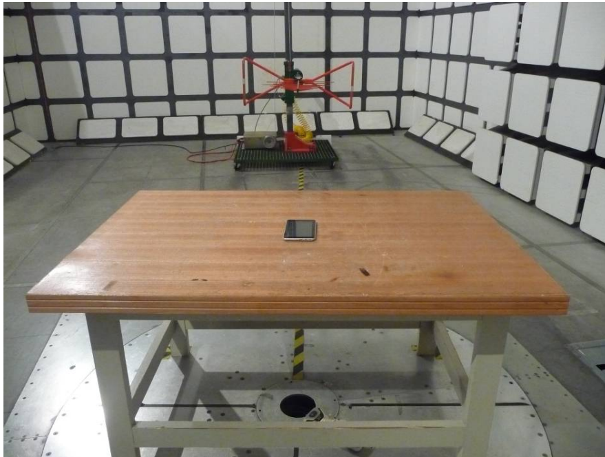
Radiated Emissions View (30-1000 MHz)
