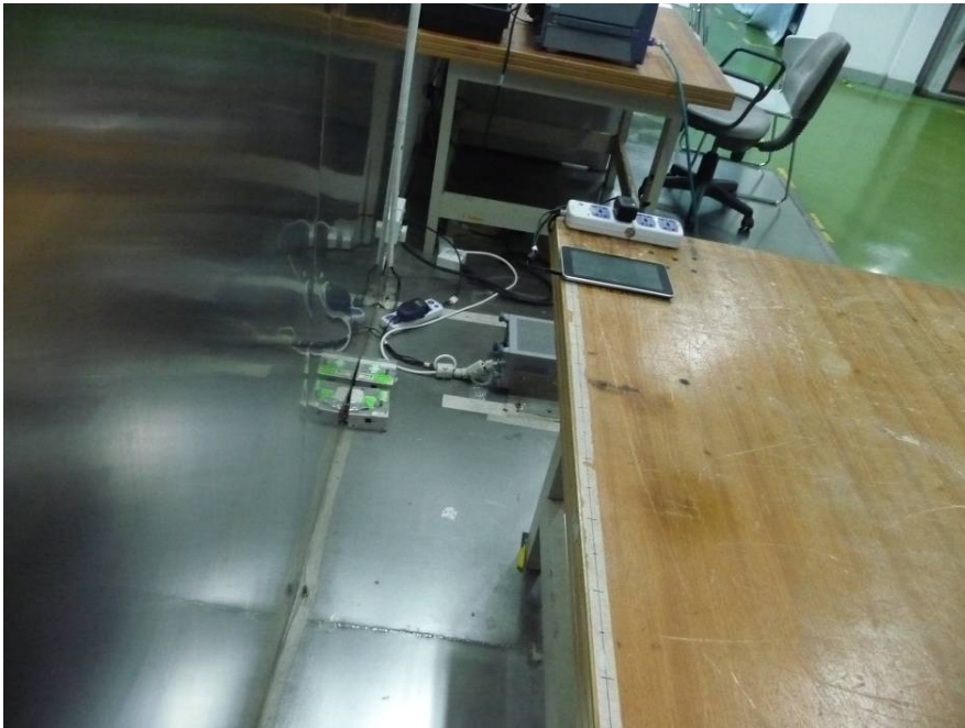
Conducted Emissions - Side View
