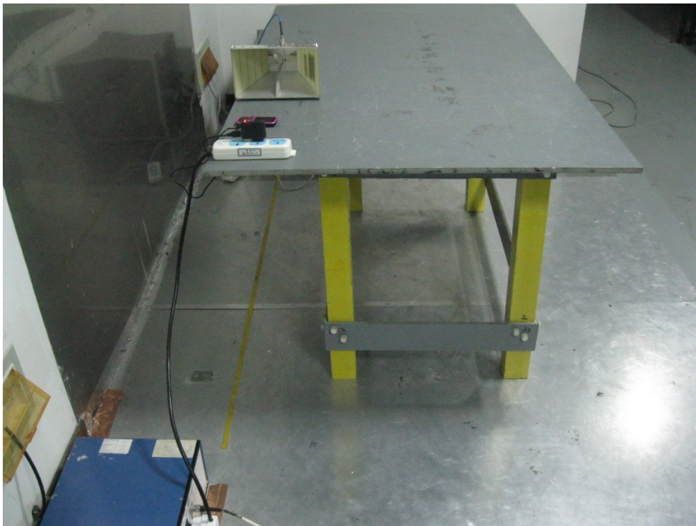
Conducted Emissions Test Setup - Side View
