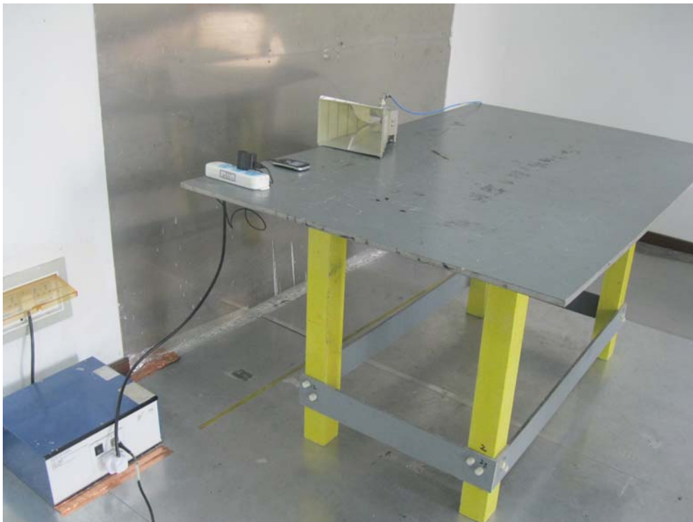
Conducted Emissions Test Setup - Side View
