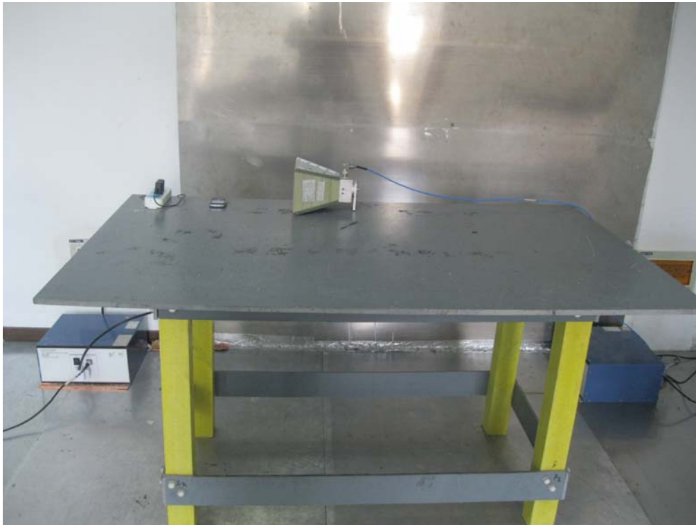
Conducted Emissions Test Setup - Front View
