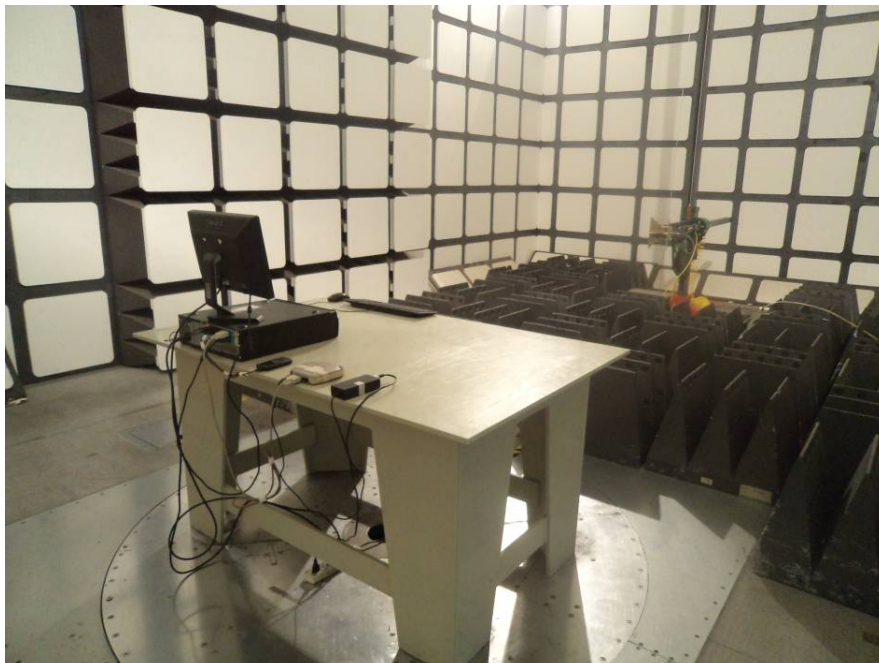
Radiated Emissions – Rear View (Above 1 GHz)
