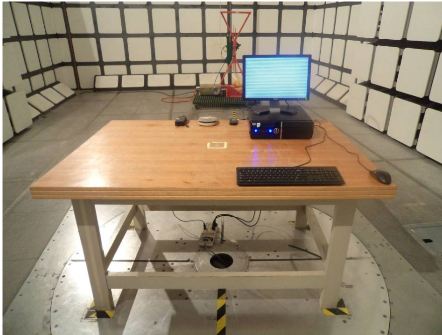
Radiated Emissions – Front View (Below 1 GHz)
