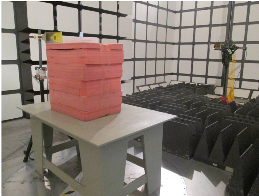
Radiated Emissions Test View (Above 1 GHz)
