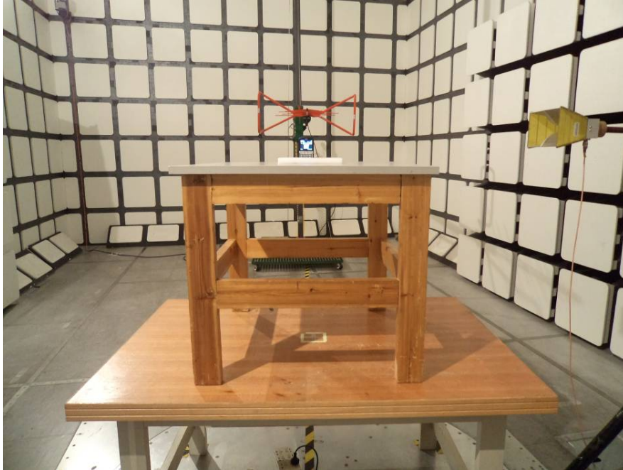
Radiated Emissions Test View (Below 1 GHz)
