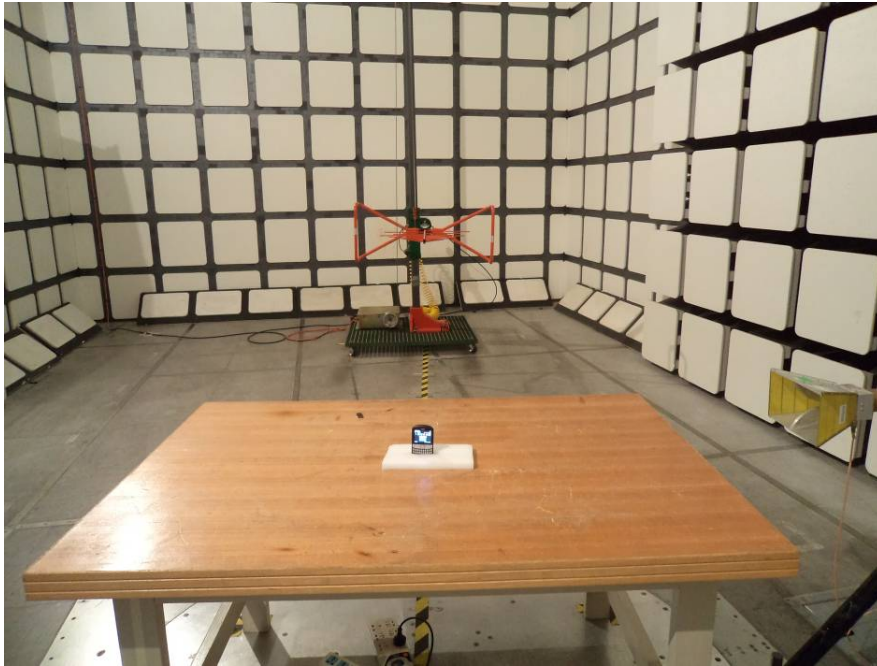
Radiated Emissions View (Below 1 GHz)
