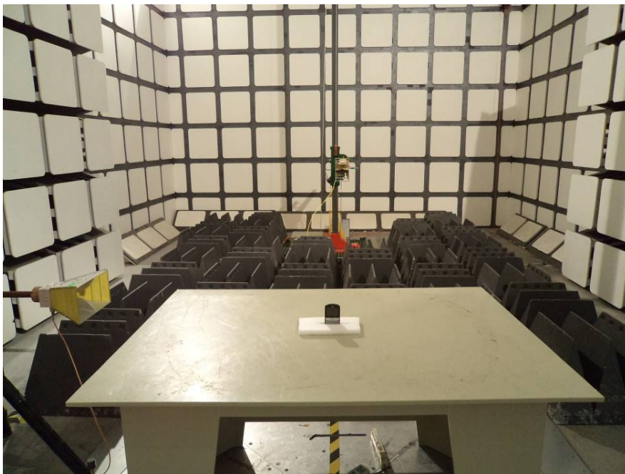
Radiated Emissions View (Above 1 GHz)
