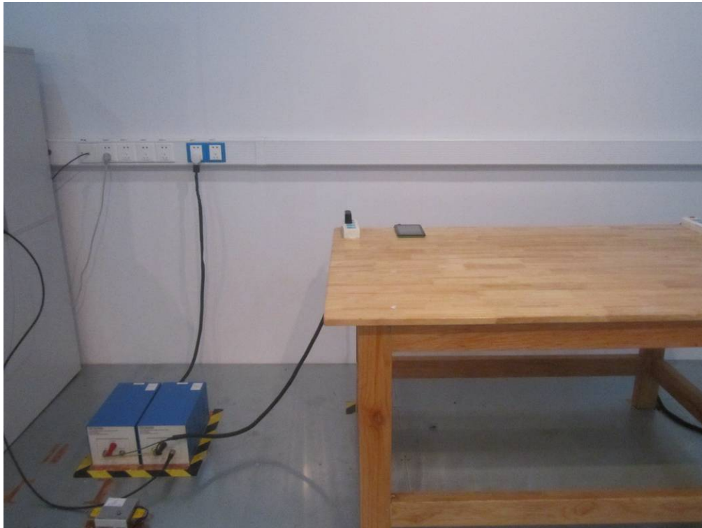
Conducted Emissions Test Setup Front View
