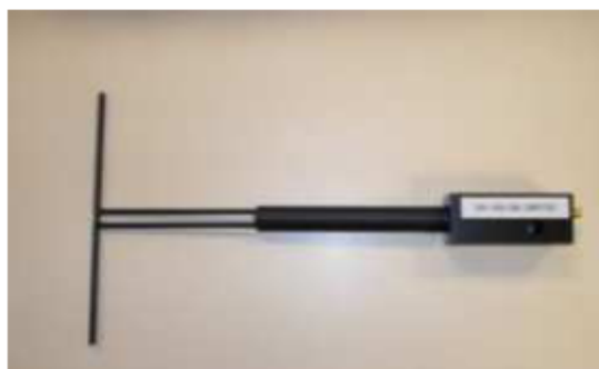
Figure 1 – Satimo COMOSAR Validation Dipole
