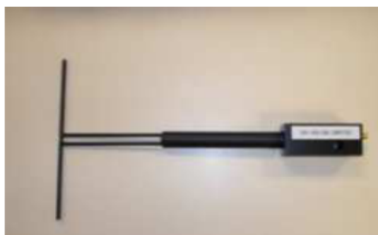
Figure 1 – Satimo COMOSAR Validation Dipole
