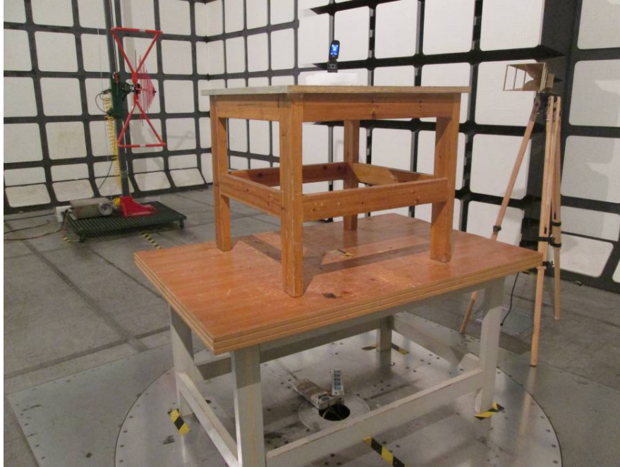
Radiated Emissions Test View (Below 1 GHz)
