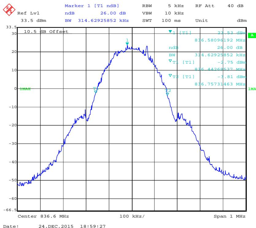
**PCS Band (Part 24E)****99% Occupied Bandwidth for GSM (GMSK) Mode**
