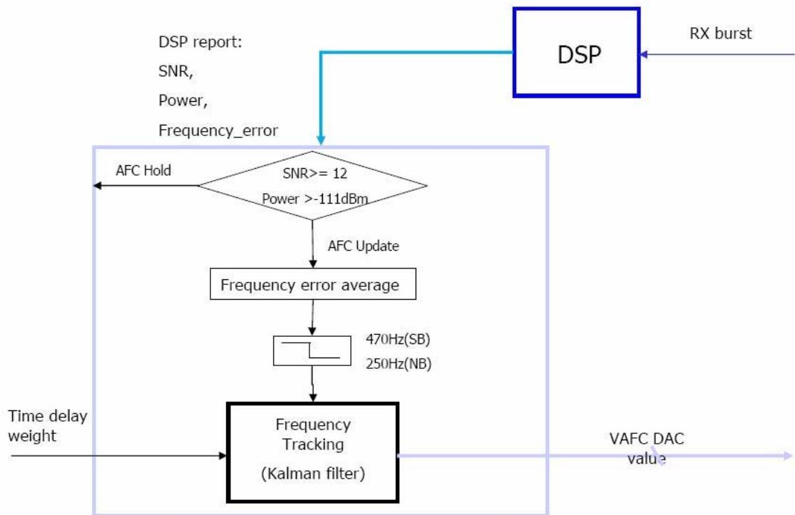
In SC6531, it uses an AFC signal from baseband (DAC) to finish automatic frequency control.
