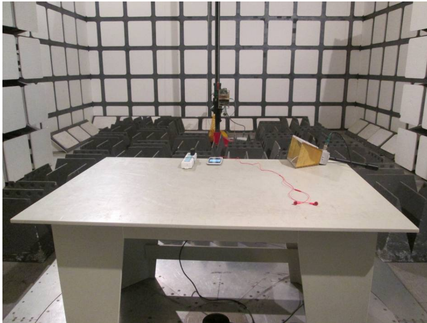
Radiated Emissions - Front View (Above 1 GHz)
