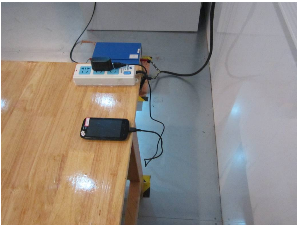
Conducted Emissions Test Setup Side View
