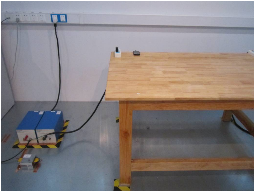
Conducted Emissions Test Setup Front View
