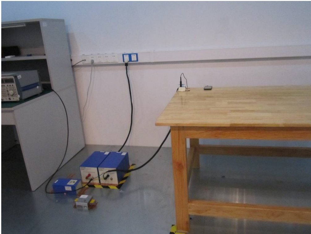
Conducted Emissions Test Setup Front View
