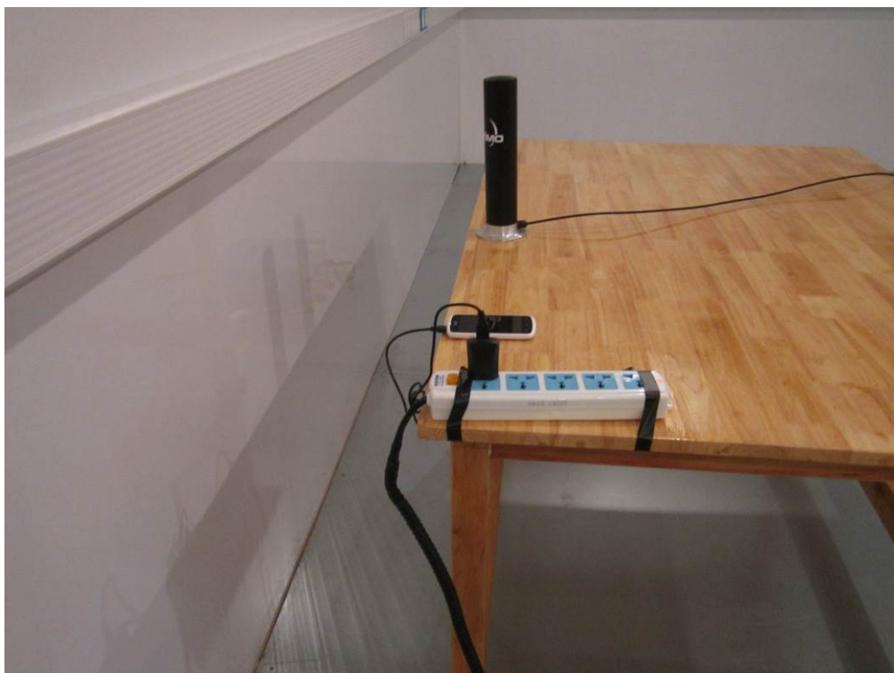
Conducted Emissions Test Setup Side View
