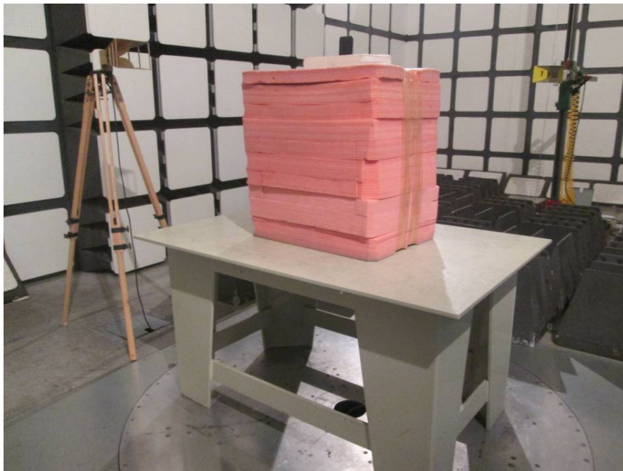
Radiated Emissions Test View (Above 1 GHz)
