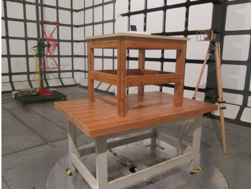
Radiated Emissions Test View (Below 1 GHz)
