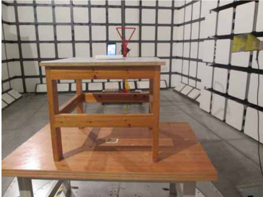
Radiated Emissions Test View (Below 1 GHz)
