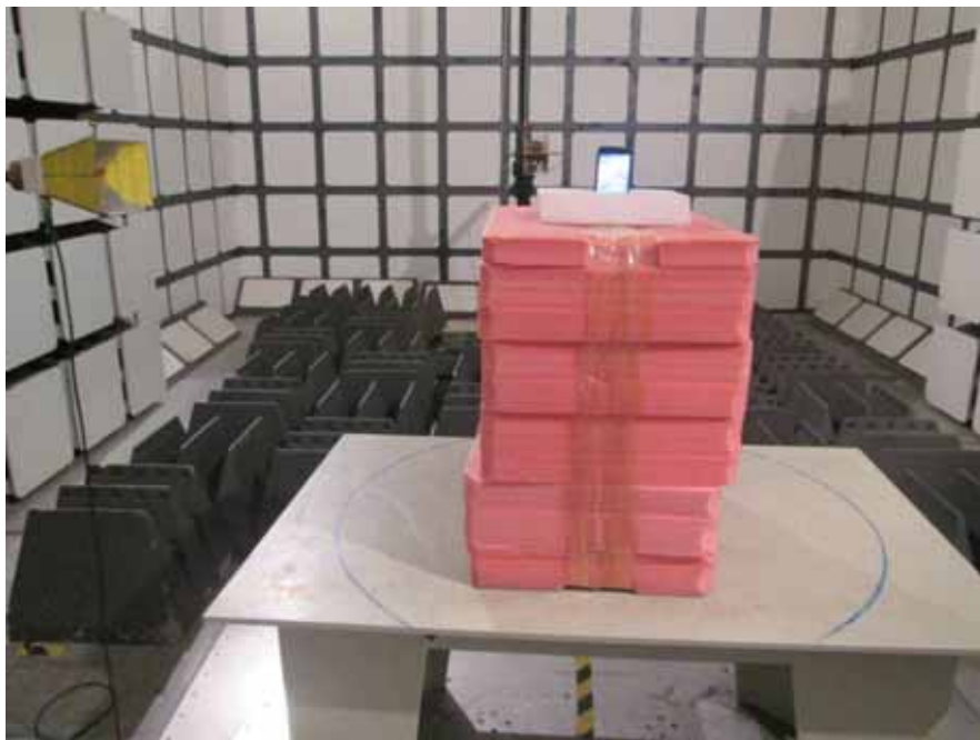
Radiated Emissions Test View (Above 1 GHz)
