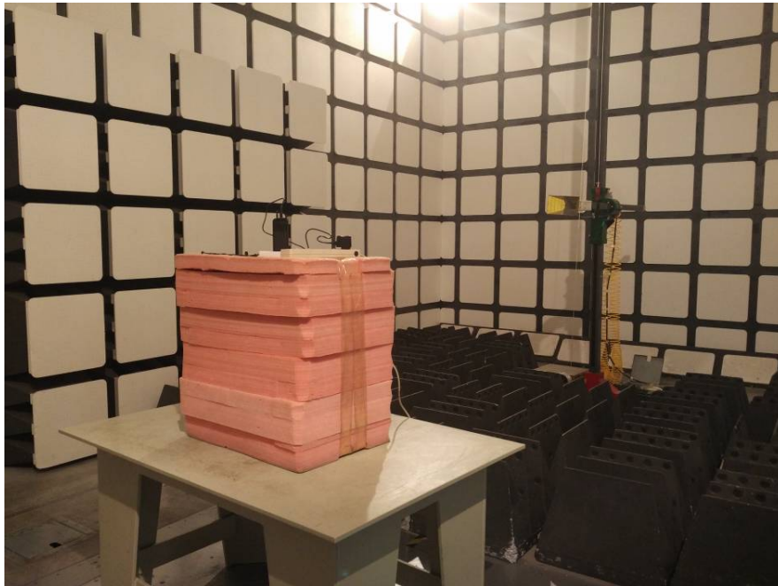
Radiated Emissions View (Above 1 GHz)
