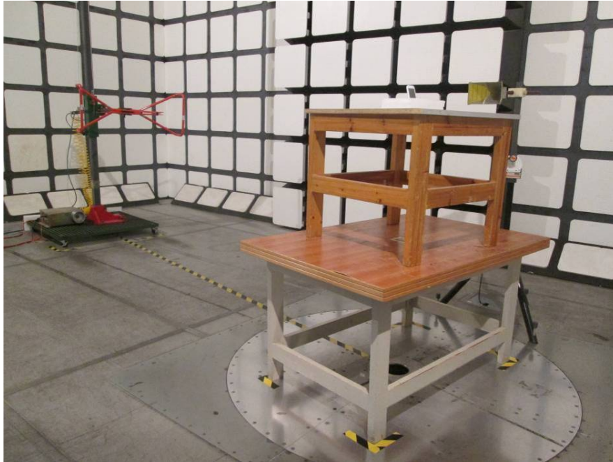
Radiated Emissions Test View (Below 1 GHz)
