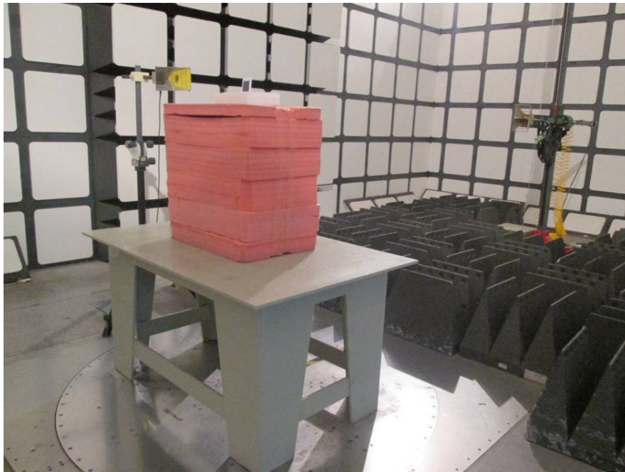
Radiated Emissions Test View (Above 1 GHz)
