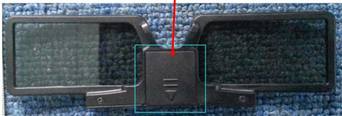
Remark: The cover of the battery box can be opened but can not be removed away from the EUT.
