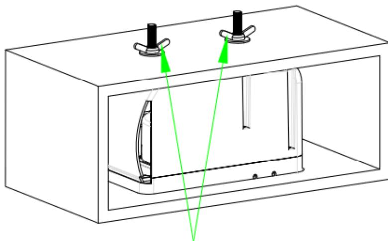
4: Install gasket and tighten nut
