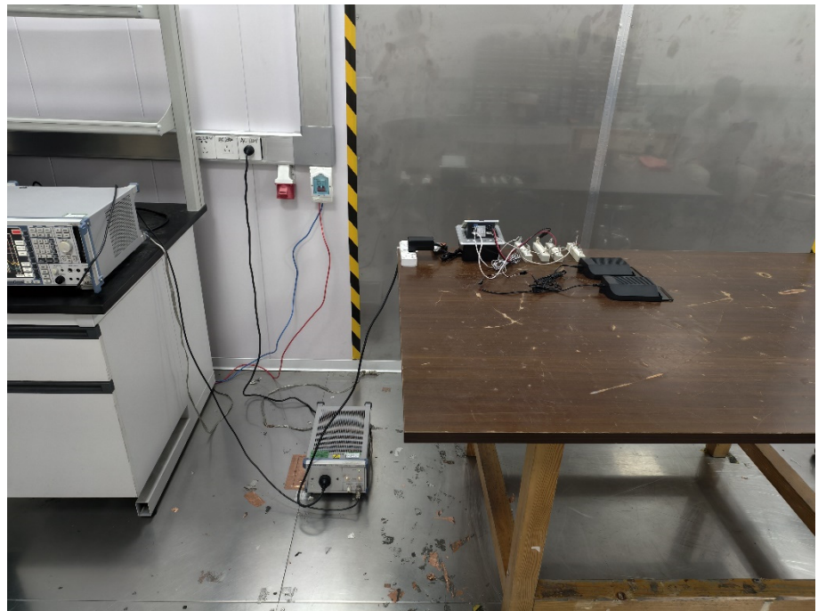
Conducted Emission Test Setup
