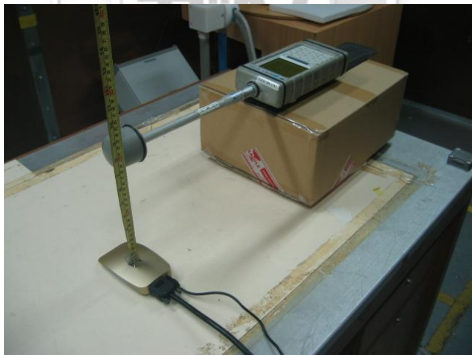
Maximum Permissible Exposure (MPE) Test Setup
