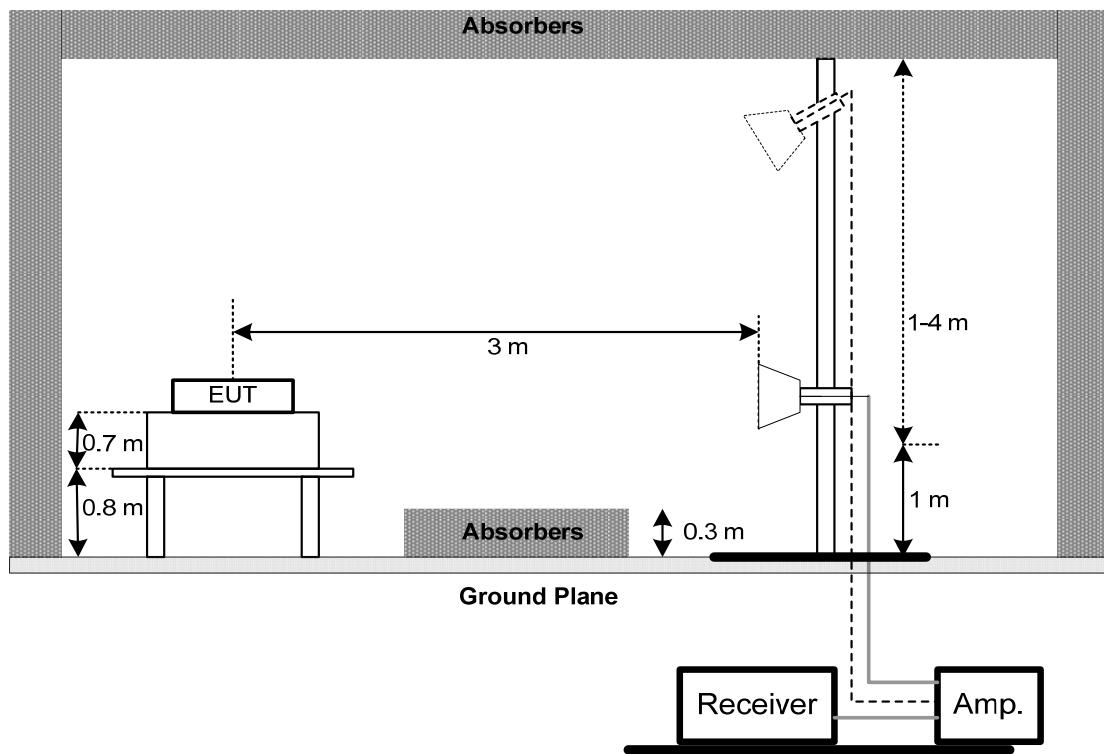
(C) For radiated emissions below 30MHz
