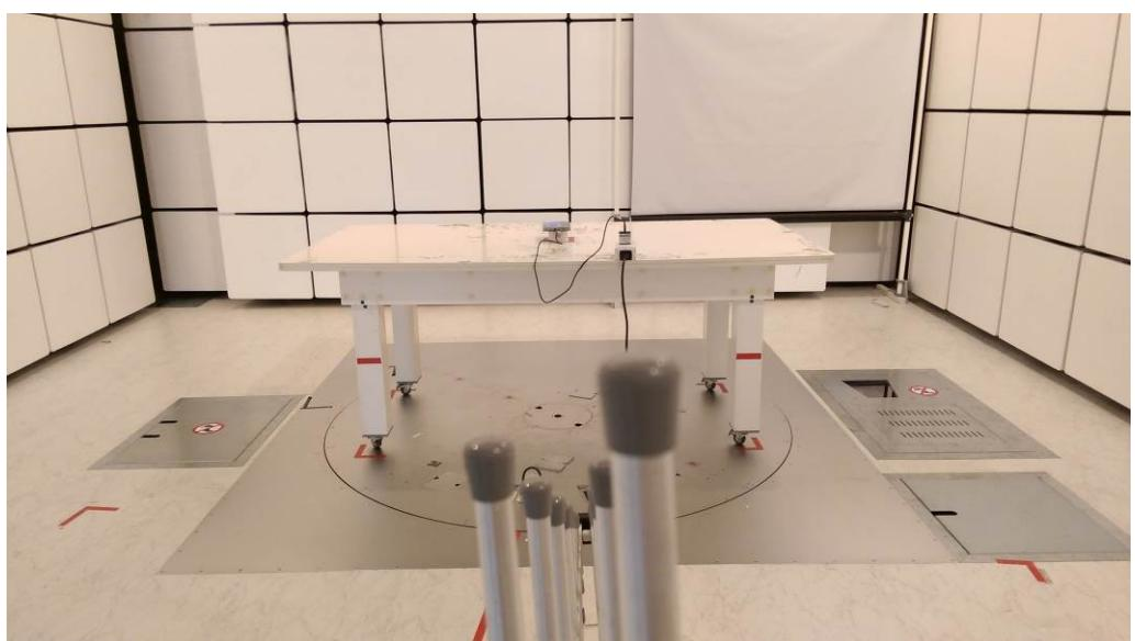
**Radiated Measurement Photos****30MHz to 1000MHz****With Smart Mount + Adapter\_DDA-18A-05 053350**
