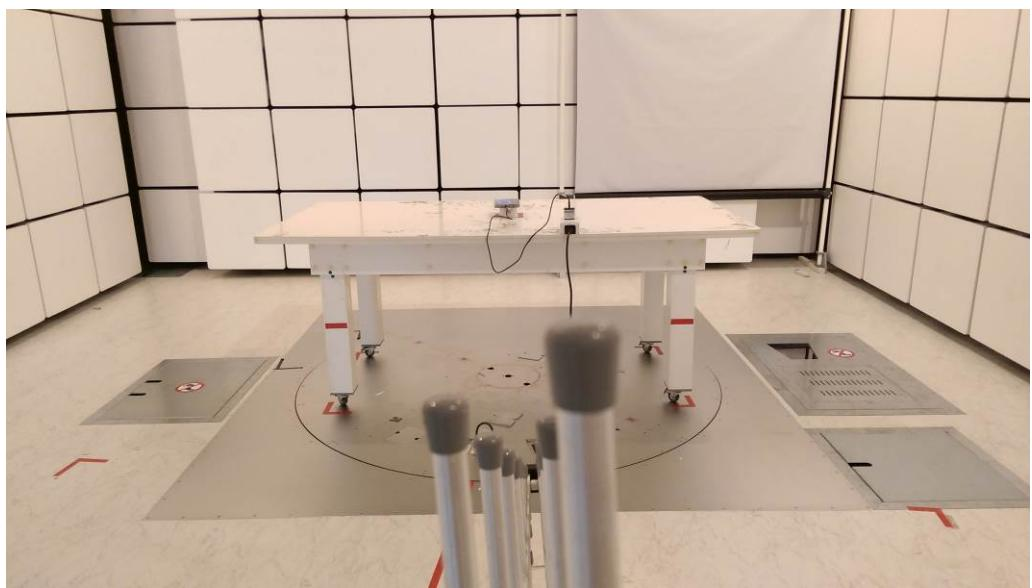
**Radiated Measurement Photos****30MHz to 1000MHz****With Smart Mount + Adapter\_DDA-18A-05 053350**
