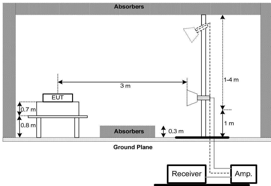
(C) For radiated emissions below 30MHz
