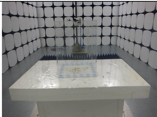
Radiated Spurious Emissions Test Setup Above 1GHz
