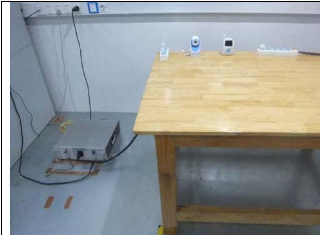
Conducted Emissions Test Setup Front View
