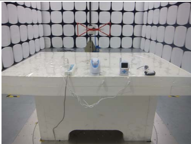
Conducted Emissions Test Setup Front View
