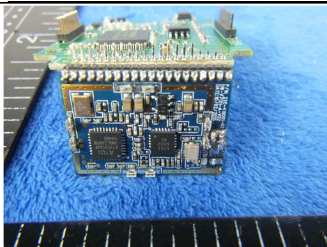
FHSS Board without shielding - Front View
