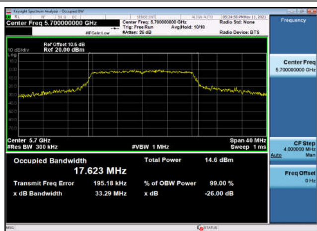
U-NII-2c 99% Bandwidth-802.11a(20MHz) ,5700MHz,Ant1
