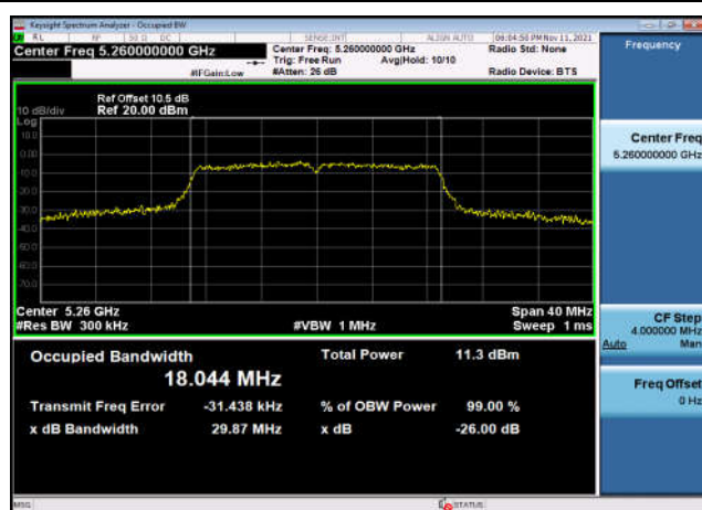
U-NII-2a 99% Bandwidth-802.11n(20MHz) ,5320MHz,Ant1
