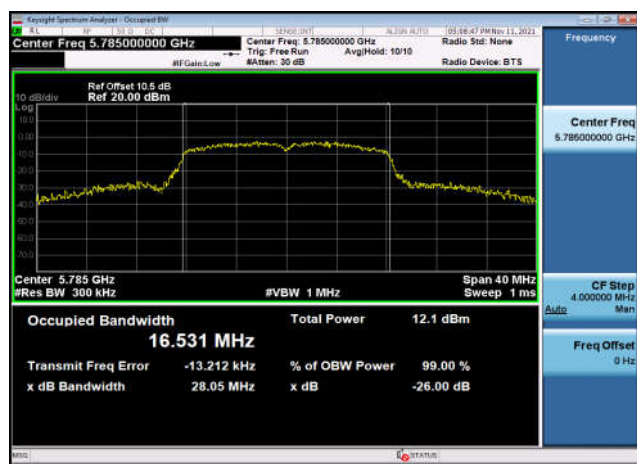
U-NII-3 99% Bandwidth-802.11a(20MHz) ,5785MHz,Ant1
