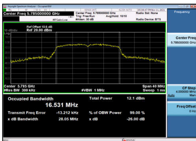
U-NII-3 26dB Bandwidth-802.11a(20MHz) ,5785MHz,Ant1
