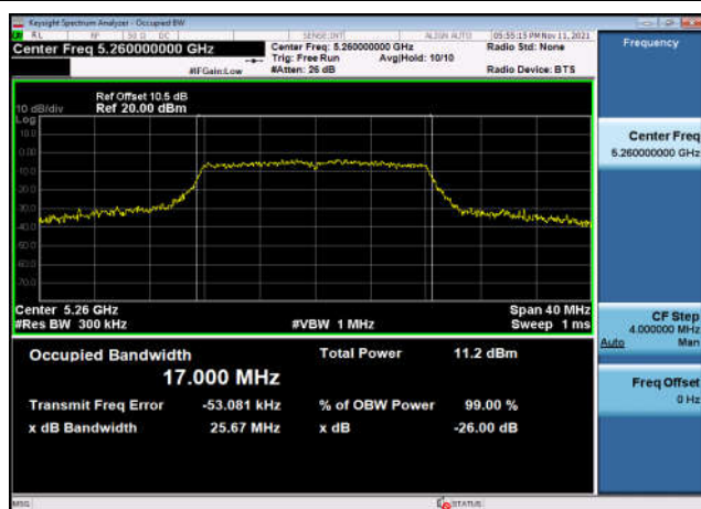
U-NII-2a 99% Bandwidth-802.11a(20MHz) ,5320MHz,Ant1
