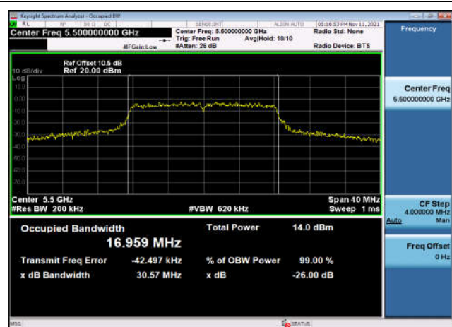
U-NII-2c 26dB Bandwidth-802.11a(20MHz ) ,5700MHz,Ant1
