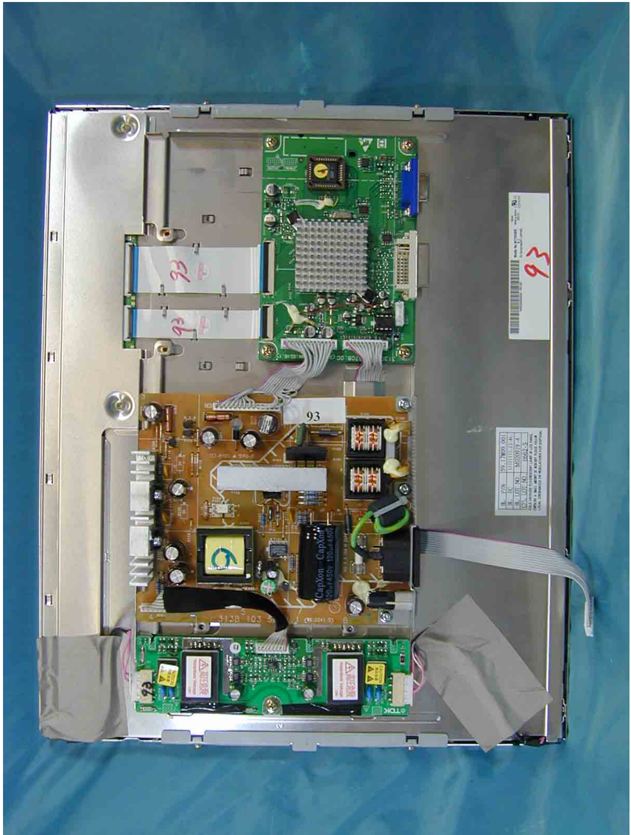
Assembly w/o Shielding Cover (AU Panel)
