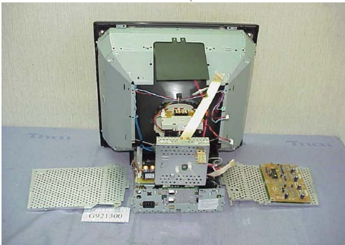
Figure 8 Display Color Monitor Internal View (Remove Drive Board & Side Shield Covers)
