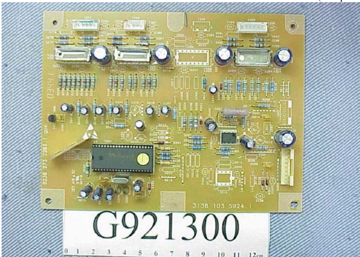
Figure 14 Display Color Monitor Drive Board (Component Side)
