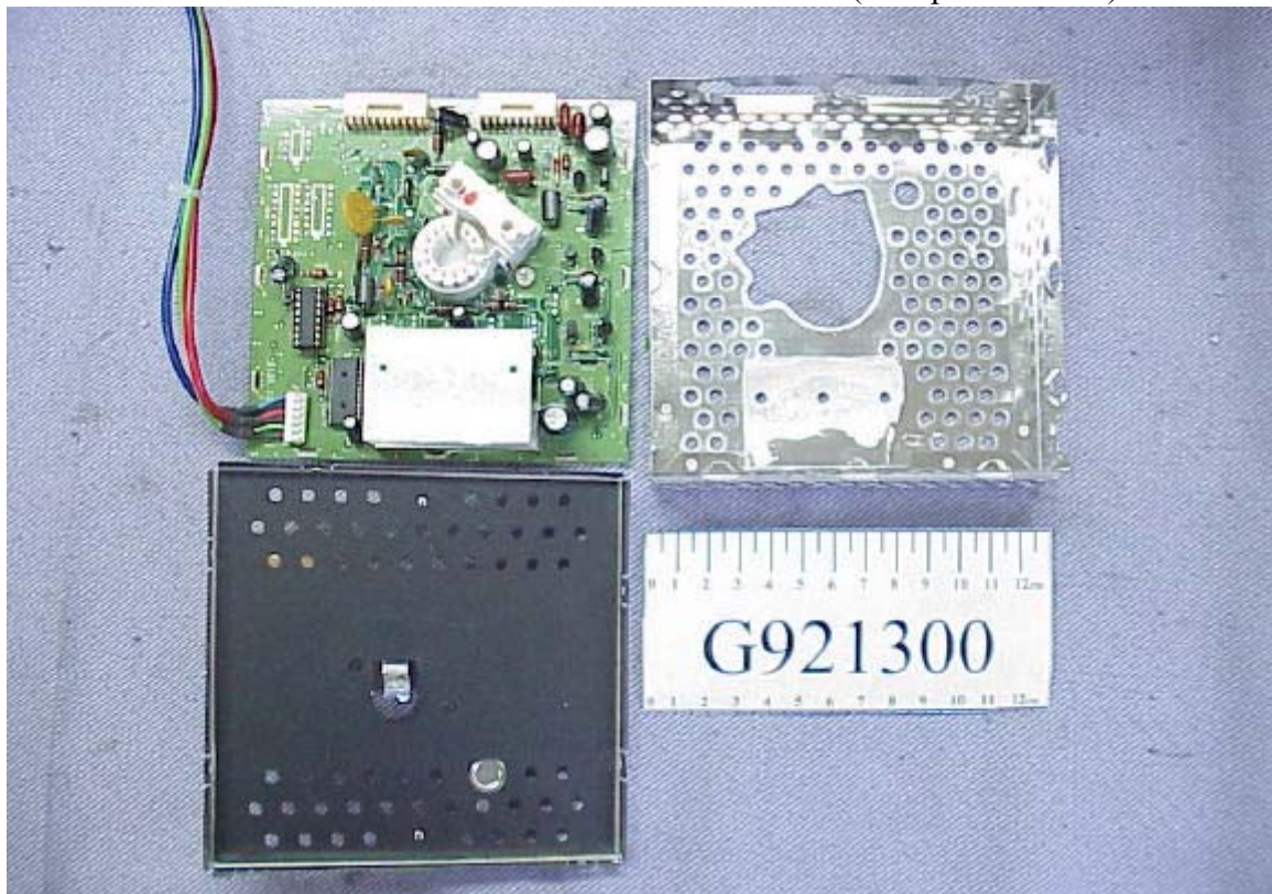
Figure 16 Display Color Monitor Video Board (Component Side) & Shield Covers
