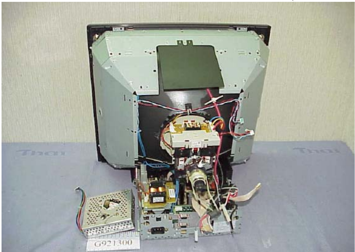
Figure 10 Display Color Monitor Internal View (Remove Video Board)
