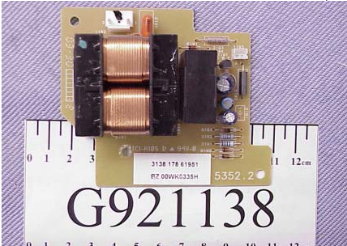
Figure 20 Display Color Monitor Transformer Board (Component View)
